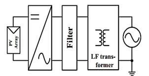
Fig. 4: Grid Side Low Frequency Transformer.
