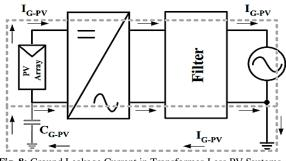
Fig. 8: Ground Leakage Current in Transformer-Less PV Systems.
