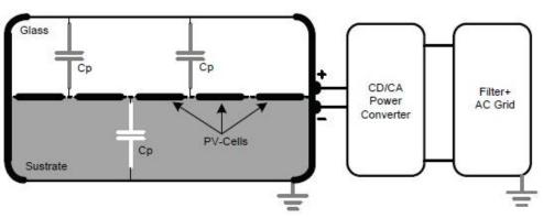
Fig. 7: Parasitic Capacitance in PV Panels.
