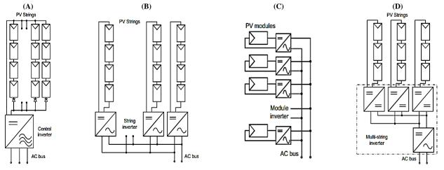
Fig. 3: Different Types of Grid-Connected PV Inverters A) Central Inverter. B) String Inverter. C) Module Inverter. D) Multistring Inverter.
