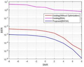
Figure 7: BER comparison based on proposed 2-dimensional 8QAM using 2×2 MIMO systems over fading channel
