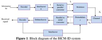
Let us consider the input information bit (B), which is transmitted through the transmitter. In the proposed approach, the sequence of M coded and interleaved bits,  $i_0, i_1, \dots, i_{M-1}$  is grouped into blocks of n×m bits, which n=log<sub>2</sub>N is the number of bits per conventional complex symbol and n is the number of dimensions. Here, we assume a number of transmitted antennas is equal to the number of dimensions. The sth block is denoted as;
