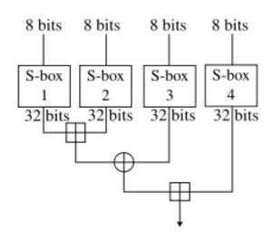
Fig. 6. Computation Performed by S-Box
