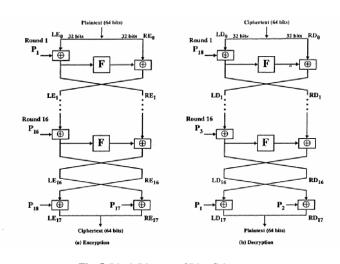
Fig. 5. Block Diagram of Blowfish
