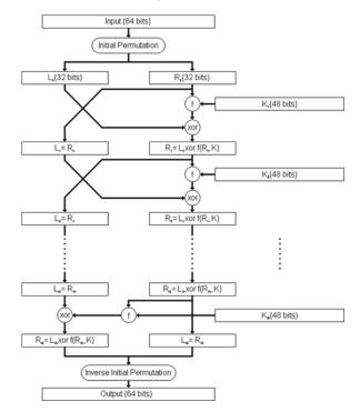
Fig. 2. Block Diagram of Triple DES
