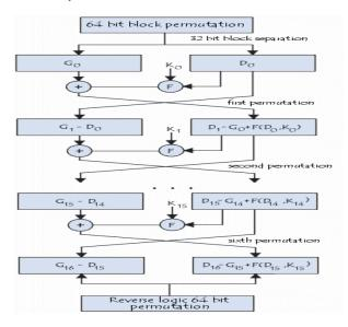
Fig. 1. Block Diagram showing working of DES
