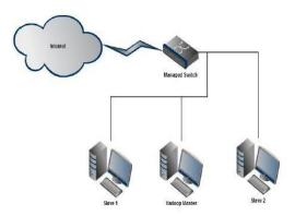
Fig. 2: Experimental Setup for Hadoop Multi-node
