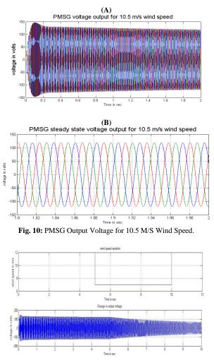
Fig. 11: Wind Velocity Is Changed from 12 M/S to 7m/S at T=5 Sec and 7 M/S to 12 M/S at T=10 Sec Respectively.
