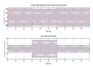
**Fig. 13:** Step Change in Load from 4 A to 9 A at T=0.3 Sec and from 9 A to 4 A at T=0.6 Sec.
