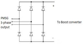
Fig. 4: Uncontrolled Rectifier.
