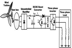
Fig. 1: Configuration of PMSG Based WEECS Feeding Isolated Load.
