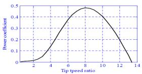
**Fig. 2:** The Relation between Power Coefficient (Cp) and Tip Speed Ratio  $(\Lambda)$  at Zero Blade Pitch-Angle.
