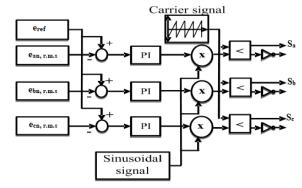
Fig. 9: PWM Generation for Unbalanced Load.
