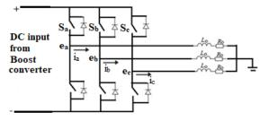
Fig. 6: Three Phase Inverter.
