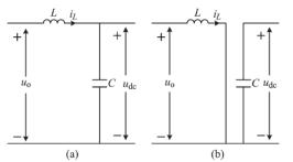
Fig. 5: Operating Modes of Boost Converter when A) Switch Turned OFF B) Switch Turned ON.
