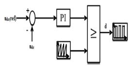
Fig. 8: Control Structure of DC-DC Converter.
