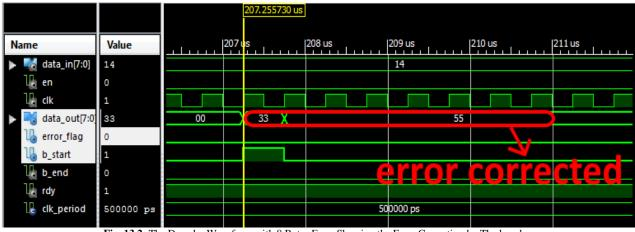
Fig. 13.2: The Decoder Waveform with 8 Bytes Error Showing the Error Correcting by Thedecoder.
