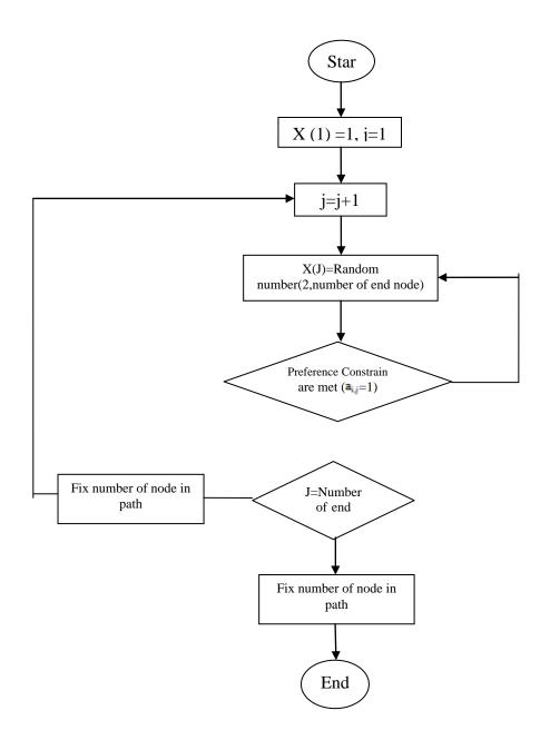
Fig.1.The proposed model of generate paths
