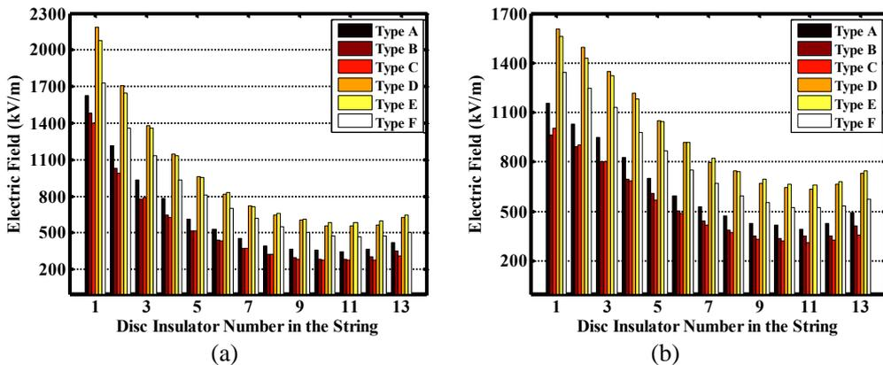
Fig. 9. Local maximums of electric field along line 1 for different insulator strings (a) without corona ring (b) with corona ring
