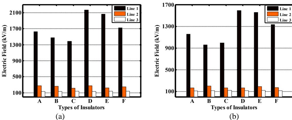
Fig. 10. Maximum values of electric field along lines 1-3 for all types of insulator strings (a) without corona ring (b) with corona ring
