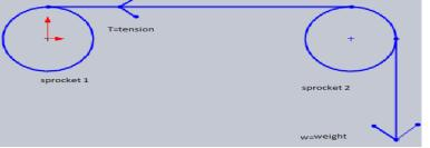
Fig. 3: Free Body Diagram of Chain.
