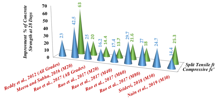
Fig. 3: The Improvement of Compressive Strength f_c' and Split Tensile Strength f_t at 28 Days in BC (at 10^5 Cells/ml B. Subtilis JC3) Concluded By Different Literature Reviews.
