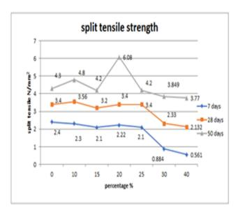
Figure 10 Split tensile strength of concrete
