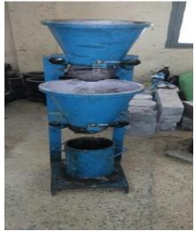
Figure 2 Compaction factor test on concrete
