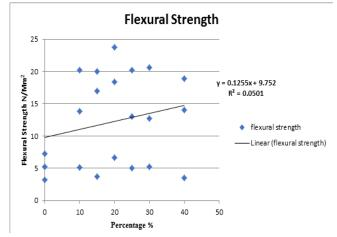
Figure 9: Flexural Strength of Concrete for various percentages of mineral admixtures
