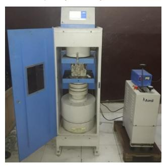
Figure 11 Split Tensile Testing Machine
