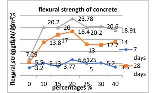
Figure 8: Flexural Strength of Concrete percentages of mineral admixtures
