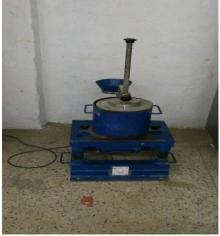
Figure 3 Vee Bee Consistometer
