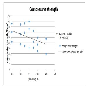
Figure 6: Compressive Strength of Concrete for various percentages of mineral admixtures
