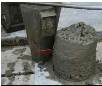
Figure.1 Slump Cone
