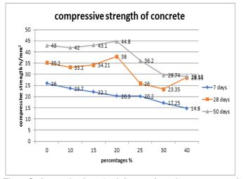
Figure 5: Compressive Strength of Concrete for various percentages of mineral admixtures
