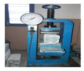
Figure 7 Flexural strength testing machine
