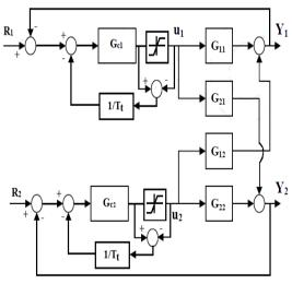
Fig. 1: Decentralized control structure with anti-reset windup
