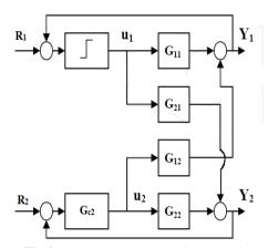
Fig. 4: Relay in loop 1 with loop 2 automated
