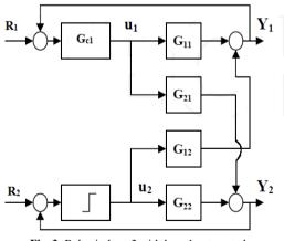
Fig. 3: Relay in loop 2 with loop 1 automated
