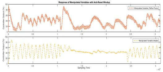
Fig. 11: Controller response with anti-reset windup
