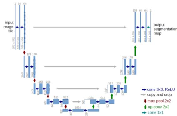
Fig. 4.1: U-Net architecture used for the generator
