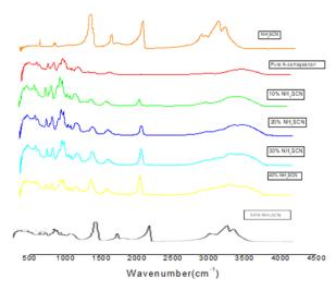
Fig. 4: FTIR spectra for varied wt. % NH<sub>4</sub>SCN
