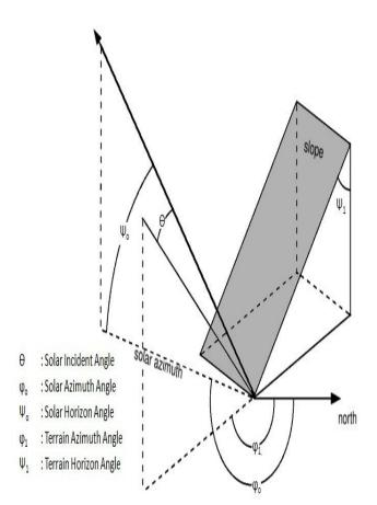
Fig. 1: Parameter involved in calculation of solar incident angle
