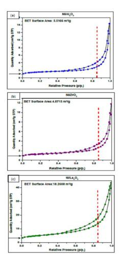
**Fig. 3**: N<sub>2</sub> adsorption-desorption isotherms of supported Ni based catalyst (a) Ni/Al<sub>2</sub>O<sub>3</sub>, (b) Ni/ZrO<sub>2</sub>, (c) Ni/La<sub>2</sub>O<sub>3</sub>
