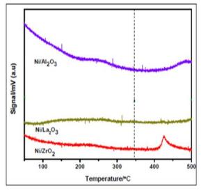
Fig.5: NH<sub>3</sub>-TPD profiles of Ni/metal oxide catalysts
