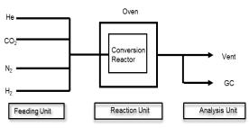
Fig. 1: Process block diagram of catalytic reactor system
