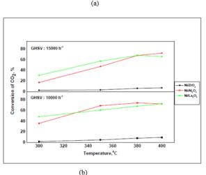
Fig. 6: (a) Conversion of  $CO_2$  over Ni/metal oxide catalysts at different temperature (b) Conversion of  $CO_2$  over Ni/metal oxide catalysts at different GHSV
