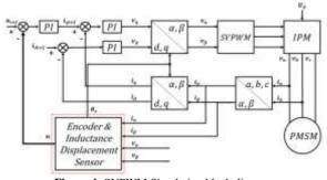
Figure 4: SVPWM Simulation block diagram
