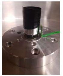
Figure 2: Encoder and Inductance Displacement Sensor
