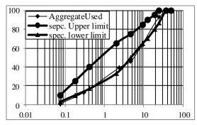
Figure 2: Gradation of Granular Material Used and Specification limits
