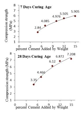
Figure 6: Effect of Adding Cement on The Compression Strength Test Rresults
