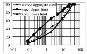
Figure 3: Corrected Gradation of Granular Material Used and Specification limits
