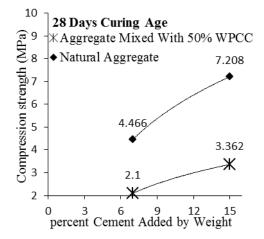
Figure 8: Effect of Using 50% WPCC in CTB on Compression Strength Test Results
