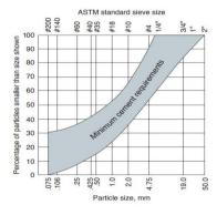
Figure 1: Minimum Cement Requirement and The Band of Aggregate Gradation(Gregory, 2006)
