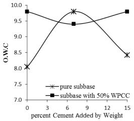
Figure 7: Effect of Using 50% WPCC in CTB on The Compaction Test results
