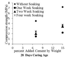
Figure 9: Effect of Soaking for Different Time Period on CTB Compression Strength Test Results
