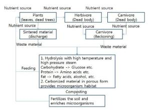
Fig.2: the concept of recycling of organic waste by high-temperature high-pressure steam
