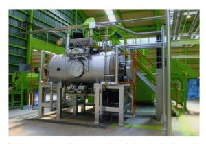
Fig.6:.High-temperature high-pressure hydrolysis carbonization equipment (AandA Ltd.)
