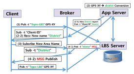
Figure 3: Converting GPS Coordinate to District Name
