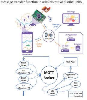
Figure 2: System Architecture and Data Flow of SLIMS
