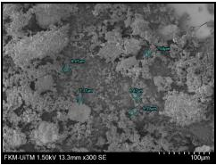
3c) Alumina Powder After using Ball Milling
