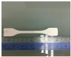
Figure 5: Mold sample after Injection
