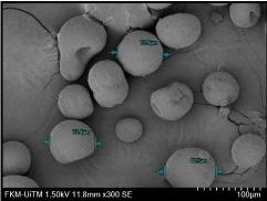
3b) Alumina powder with size range 70-150 µm
