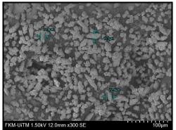
3a) Zirconia powder with size range 8-15µm
