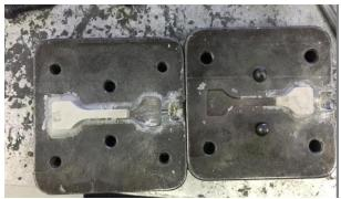
Figure 6: Crack occur after injection molding
