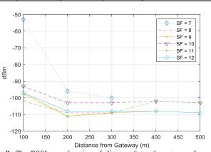
Fig. 9: The RSSI as a function of distance from the gateway for ever Spreading Factor used in the experiment
