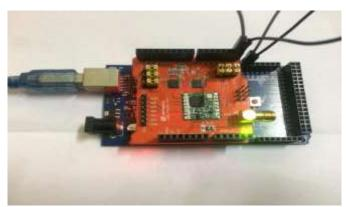
Fig. 4: DRAGINO Shield with Arduino MEGA 2560.
