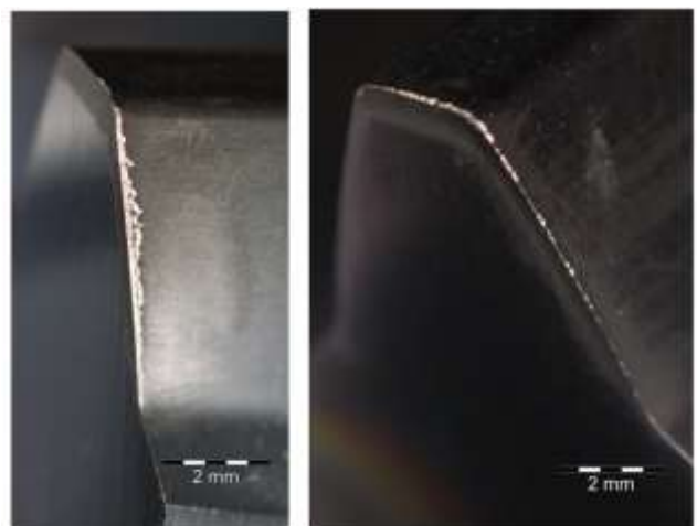
Fig.6: Wear of cutting edge with initial rounding radius R=11.18 µm (left image), R=20.12µm (right image)
