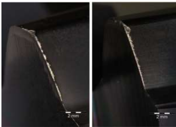
Fig.7: Wear of cutting edge with initial rounding radius R=16.13\mu\text{m} (left image), R=23.93\mu\text{m} (right image)
