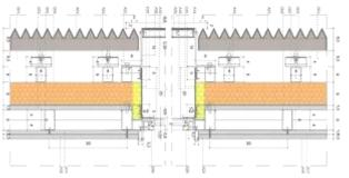
**Fig. 6:** Detail of the horizontal section of the façade. (a) Current solution. (b) Solution proposed with ceramic pieces.
