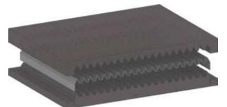
Fig. 4: Pressing the large-format ceramic piece and 3.5 mm thick.
