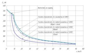
**Fig. 3:** The traction characteristics of the shunting diesel locomotive of the ChME3 series and the hybrid on its base.
