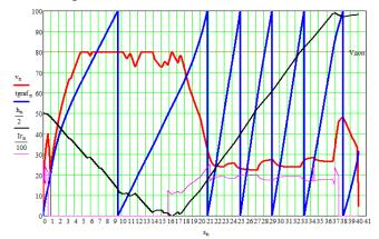
Fig. 4: Traction calculations of diesel locomotive of ChME3 series, which moves with a train of mass 500t by profile Stakhanov-Popasna:  $v_n$  – speed curve, km/h; tgraf<sub>n</sub> – curve of time running, min;  $h_n/2$  - profile of the train motion section,  $I\Gamma_n/100$  – current curve, A,  $s_n$  – path of the train, km.
