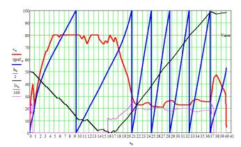
Fig. 5: Traction calculations of the hybrid diesel locomotive on the basis of ChME3, which moves with a train of mass 500t by profile Stakhanov-Popasna:  $v_n$  – speed curve, km/h;  $tgraf_n$  – curve of time running, min.;  $h_n/2$  – profile of the train motion section,  $I\Gamma_n/100$  – current curve, A;  $s_n$  – path of the train, km.
