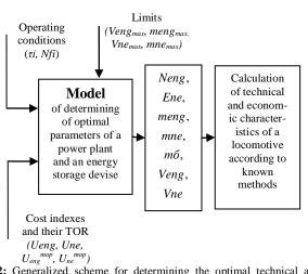
Fig. 2: Generalized scheme for determining the optimal technical and economic performance of a hybrid shunting diesel locomotive:
