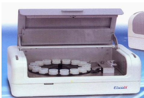
Fig. 3: X-ray fluorescence spectrometer ElvaX 3.
