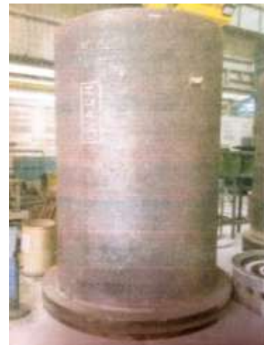
Fig.6: Rotorpost after welding
