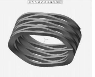
Fig.2: CADD Model of wave spring in CREO
