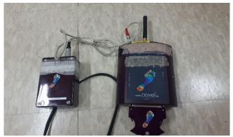
Fig.1: Battery and data transmitter of the novel pedar-x measurement system.
