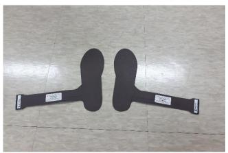
Fig.2: Insoles with built-in foot plantar pressure sensors
