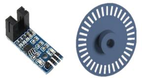
Fig. 6: (a). Infrared sensor (Left) (b). Encoder disc (Right)
