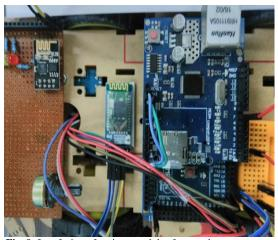
Fig. 9: Interfacing of various modules for speed measurement
