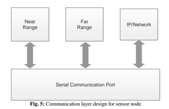
The objective of the work is to create a reconfigurable interface for different sizes of the motor or other rotating elements. The design is done with a limited data processing ability for observation, estimation, and transmission. The node has a unique identification, radio frequency link, and TCP/IP stack.
