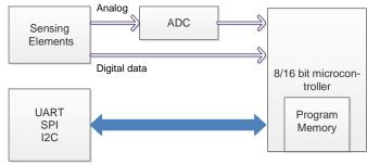
Fig. 3: Hardware design part for the sensor node
