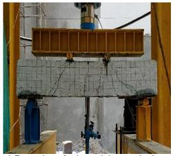
Fig. 6: Test specimen of optimum mix in conventional concrete
