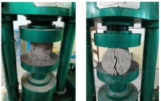
Fig. 2: Compression and Split Tensile strength testing of specimens
