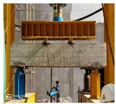
Fig. 7: Test specimen of nominal mix in SCC concrete
