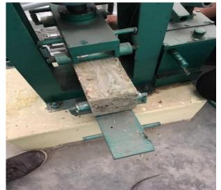
Fig. 3: Flexural testing of PCC beam specimens
