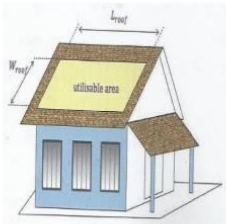
Fig.6: Possible location of PV array
