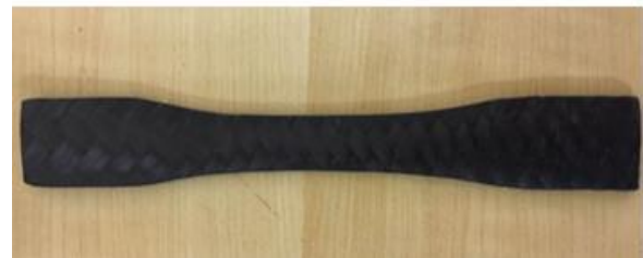
Fig. 4: The Tensile Specimens, 3.5 Mm Thick.
