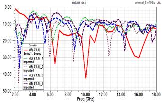
Fig. 3: Plot showing return loss enhancement over upper frequency bands through the five stages of evolution
