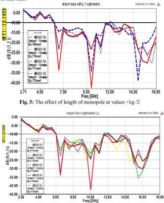
Fig. 6: Stub length tuning from Ls 11to14mm effect on antenna return loss characteristics
