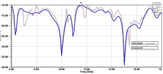
Fig. 7: Return loss plot of the simulated and fabricated antenna
