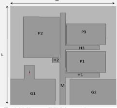
Fig. 1: Multi-octave CPW fed monopole antenna
