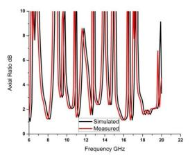
Fig. 8: Axial ratio of the simulated and fabricated antenna.
