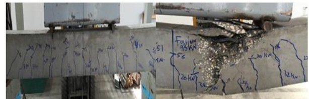
Fig. 8: The Load Displacement Curve of the Control Beam F-C and Its Crack Pattern.
