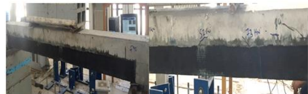
Fig. 5: Strengthening Details of Specimen F-90 that was Partially Wrapped Perpendicular to the Longitudinal Axis of the Beam.
