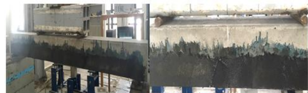
Fig. 4: Strengthening Details of Specimen F-60 that was Partially Wrapped with CFRP Inducing Angle of \pm 60^\circ to the Longitudinal Axis of the Beam.
