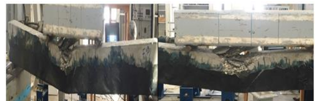
Fig. 12: The Load Displacement Curve of Beam F-45 and Its Crack Pattern.
