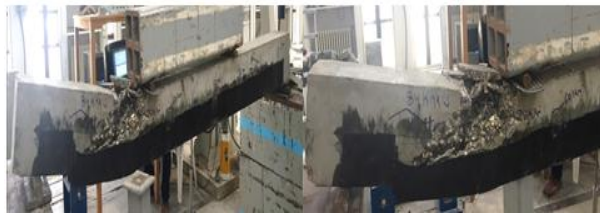
Fig. 10: The Load Displacement Curve of Beam F-90 and Its Crack Pattern.
