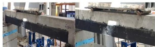
Fig. 6: Strengthening Details of Specimen F-0 that was Partially Wrapped with CFRP Parallel to the Longitudinal Axis of the Beam.
