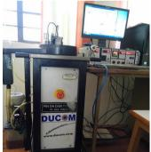
Fig. 5: Pin on disc wear testing machine
