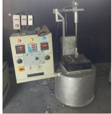
Fig. 2: Stir casting apparatus
