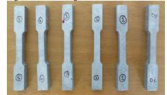
Fig. 4: Specimen of AA/FA/B as per ASTM E8M04 for Tensile test
