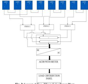
Fig. 2: Layout of Two-20kwp Solar Power Plant.
