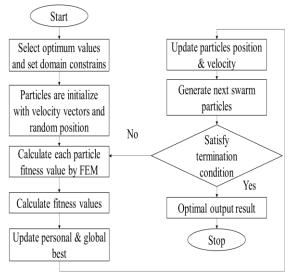
Fig. 1: Optimization design flow-chart using PSO-FEM
