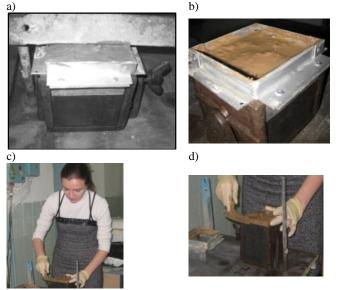
Fig. 1 Formation of soilcement samples in the form with additional attachment: a) - the beginning of creation, b) - the completion , c, d) - cuting of soilc ment remains
