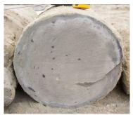
Fig. 8 Digested experimental cement piles after 28 days after placement: a - the excavated piles; b - a cut of the excavated pal, which was checked.
