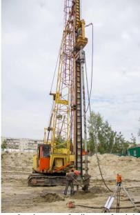
**Fig.4** Equipment for placement of soilcement foundations with high-frequency deep vibrating: a - RDK-250 with hinged drilling equipment;
