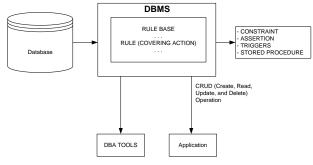
Fig. 2: Active Database Architecture
