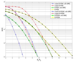
Fig. 4: BER Comparison of 8-PSK System and 8-PSSK System in Rayleigh Fading Channel.
