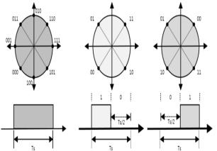
Fig. 2: Constellation and Symbol Duration for (A) 8-PSK and (B) 8-PSSK.
