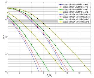
Fig. 3: BER of 8-PSK System and 8-PSSK System in Rician Fading Channels.
