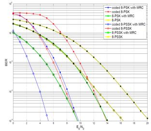
**Fig. 5:** BER Comparison of 8-PSK System and 8-PSSK System in Rician Fading Channel (K=9).
