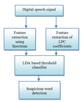
Fig. 1: The Block Diagram of Proposed Methodology
