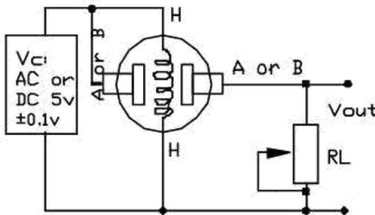
Fig. 2: MQ 7 sensor
