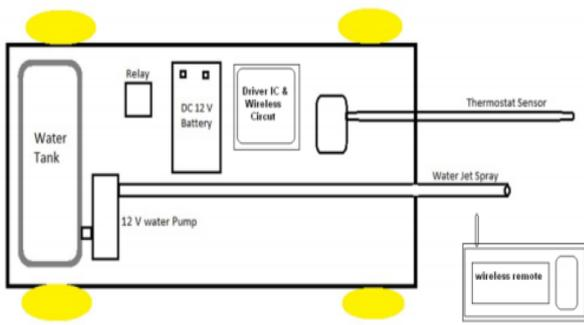
Fig. 1: Automatic fire fighting robot architecture
