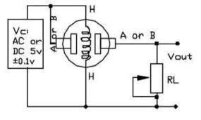
Fig. 2: MQ 7 sensor
