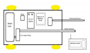
Fig. 1: Automatic fire fighting robot architecture
