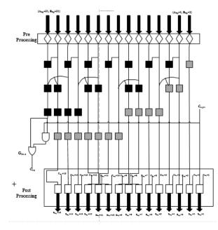
Fig. 2.7 Internal structure of Sklansky cska
