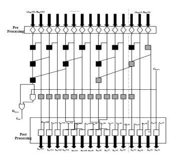
Fig. 2.2: Internal structure of Brent Kung cska
