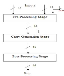
Fig. 2.3: Structure of Brent-Kung adder
