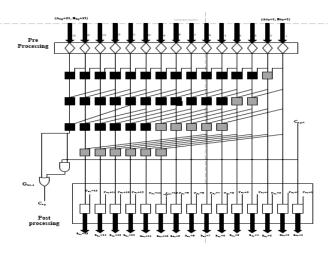
Fig. 2.5: Internal structure of Kogge-Stone cska
