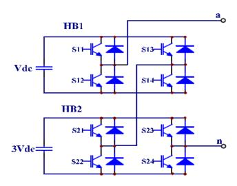
Fig. 1: MLI using Trinary DC source
