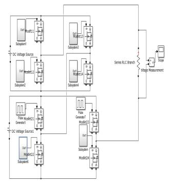
Fig. 3: Simulink model of 9-level Trinary source MLI
