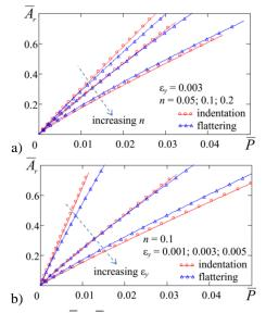
**Fig. 1.** Dependencies  $\overline{A}_r - \overline{P}$  for different values of hardening parameters.
