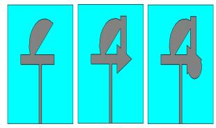
Fig. 5: Geometry of the Proposed Antennas (A) Antenna1 (B) Antenna2 (C) Antenna3.
