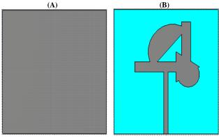
Fig. 1: Proposed Antenna Geometry (A) Back Side (B) Front Side.
