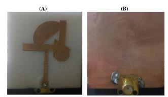
Fig. 7: Hardware of Anticipated Antenna 3 (A) Front Side (B) Back Side.
