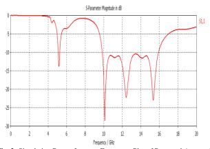
Fig. 2: Simulation Return Loss vs. Frequency Plot of Proposed Antenna3.
