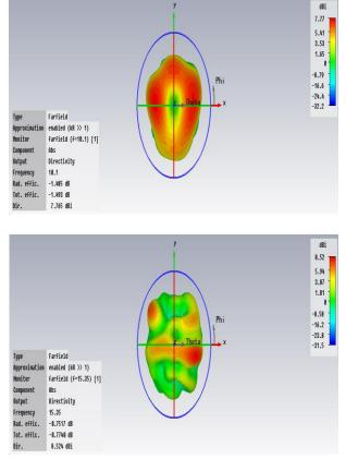
Fig.4: 3D Pattern of Presented Antenna at 10.1 GHz and 15.35 GHz.
