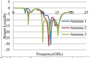
Fig. 6: Return Loss vs. Frequency of Antenna1, Antenna2 and Antenna3.
