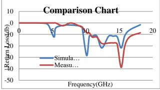
Fig. 8: Similarity of Simulated and Measured Return Loss Plot of Proposed Antenna3.
