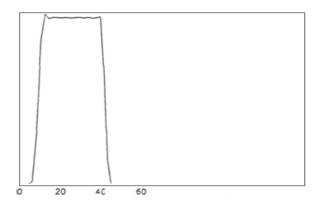
Fig. 1. Symmetrical Ormsby wavelet along vertical line.
