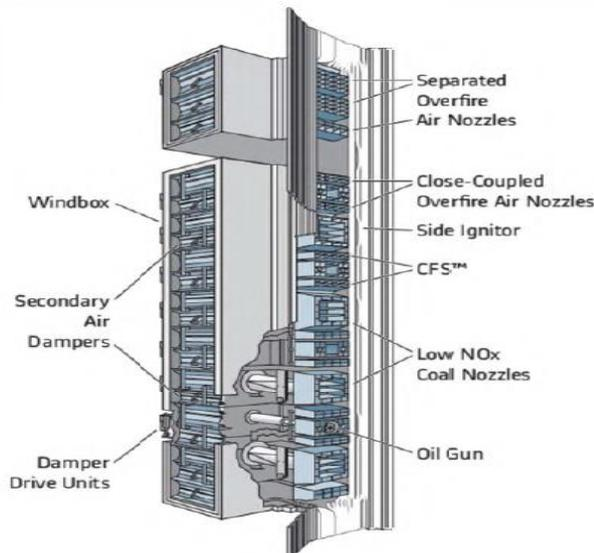
Fig. 1: Windbox and SADC
